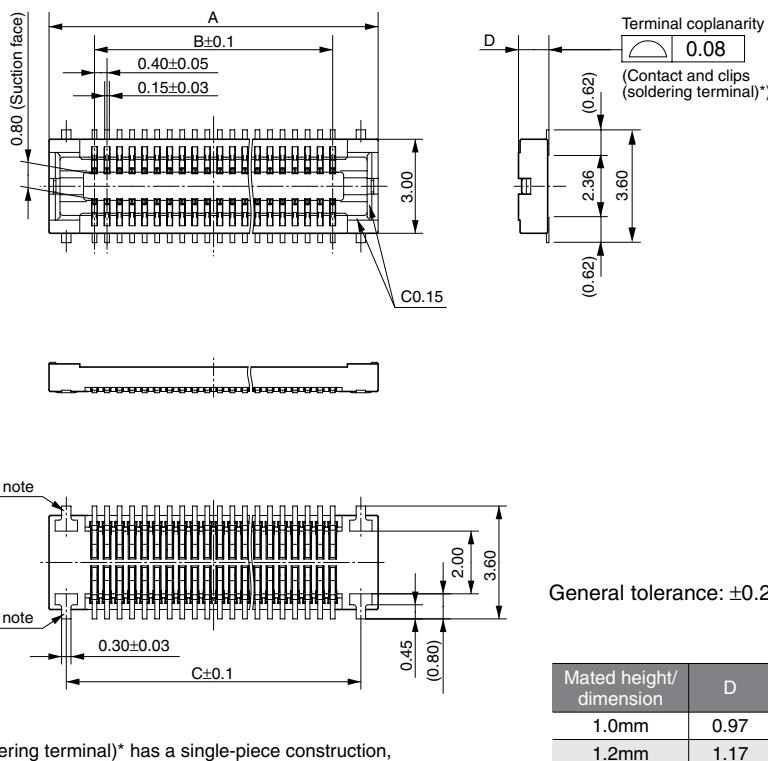
Note: Since the clip (soldering terminal)\* has a single-piece construction, sections Y and Z are electrically connected.
