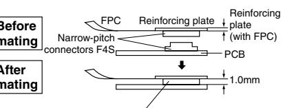
The simple lock mechanism ensures that the connector clicks into position when it is inserted for reliable single-action insertion on the PCB.
